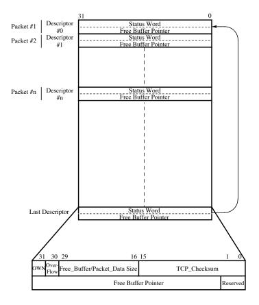
Figure 11. Receive Host Data Structure
